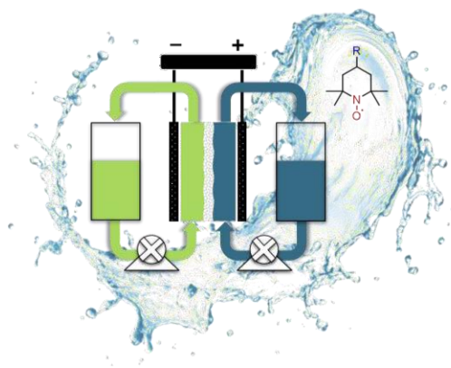
Figure 1. Schematic representation of a nitroxide-based aqueous organic redox flow battery (AORFB) and its envisioned application for grid-scale storage coupled to renewable energy sources.
